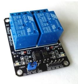
Gambar 2.5. Modul Relay 2 Channel
