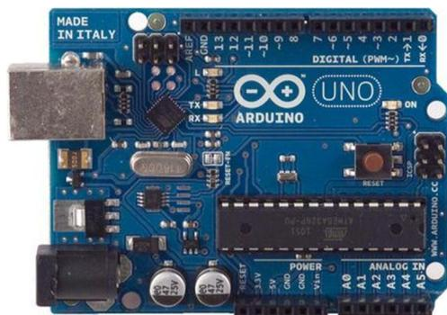
Gambar 5: Board Arduino Uno
