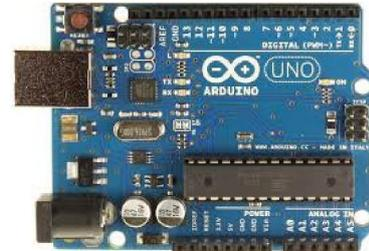
Gambar 1: Arduino Uno Board
